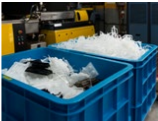
Recycling material diverted from the waste stream during a manufacturing processes such as extrusion
