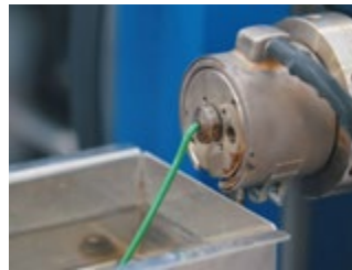
During extrusion, filament is laser-measured to ensure \pm 0.05 mm diameter tolerance and a minimum of 95% roundness
