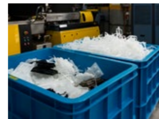
Recycling material diverted from the waste stream during a manufacturing processes such as extrusion
